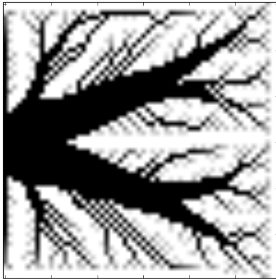
Fig. 3: Visualization of the solution for a topology optimization problem on heat diffusion, using a 60 by 60 grid for the FEM simulation
