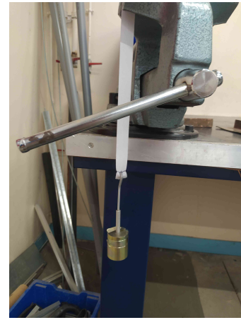
Fig. 3: Elastic band testing setup
