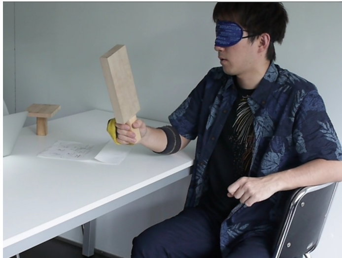
Fig. 1: Experimental setting: the subject is holding the handle of the object and wears two straps containing the IMUs sensors.
