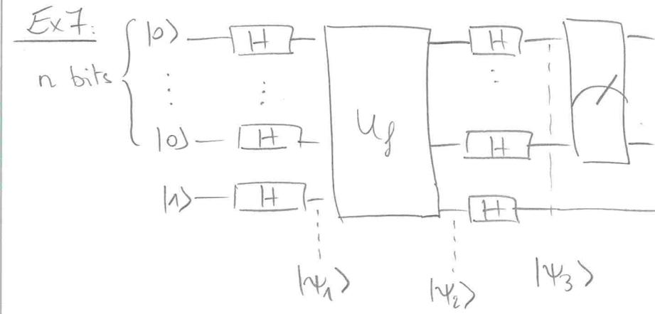
$$|\Psi_1\rangle = \frac{1}{\sqrt{2}}(|10\rangle + |11\rangle) \otimes \dots \otimes \frac{1}{\sqrt{2}}(|10\rangle + |11\rangle) \otimes \frac{1}{\sqrt{2}}(|10\rangle - |11\rangle)$$
